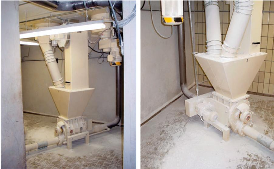
Figure 4: Inlet of a pneumatic conveying system
