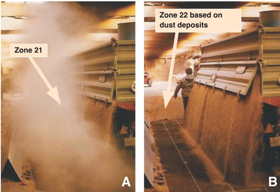
Figure 5: Discharge of corn from a truck
