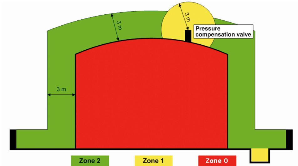
Figure 17: Area classification drawing for an external storage tank with a fixed roof containing highly flammable liquid [10]
