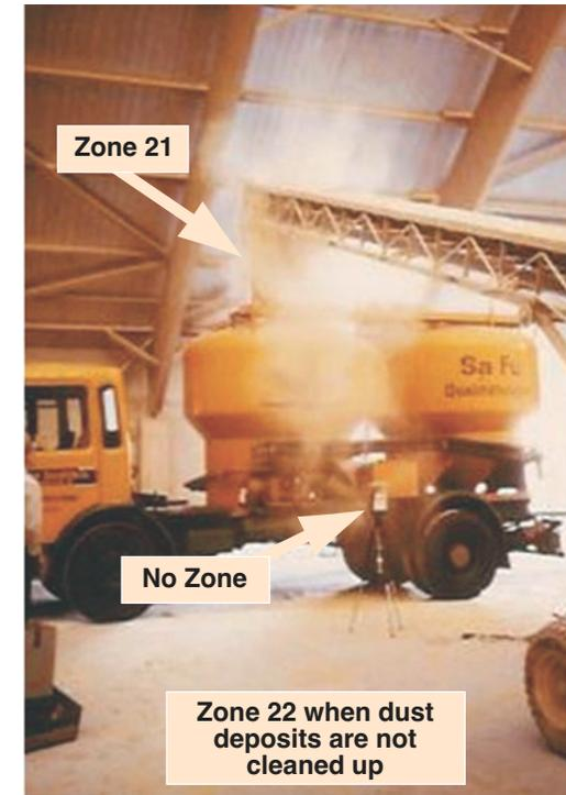
When a silo truck is filled with corn seed using an open conveyor belt as shown in Figure 6, the lower explosion limit is not exceeded except in the close vicinity of the discharge point. A zone is not allocated to the area beyond the discharge point provided that the area is cleaned each shift (elimination of dust deposits).
