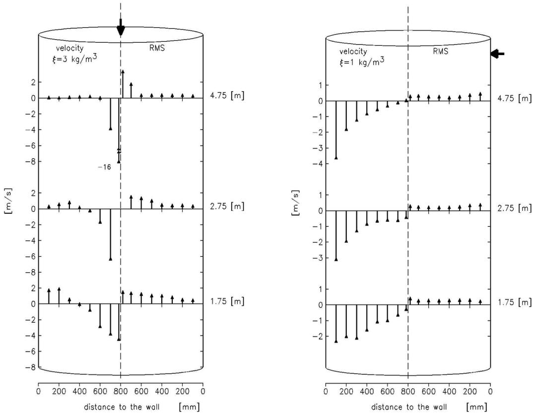
**Figure 4:** (a) The left side shows the flow velocity, the right side shows the RMS turbulence velocity of the component in z-direction at a feeding rate of  $3 \text{ kg/m}^3$  and vertical filling ( $v_c=\text{max}$ ).
