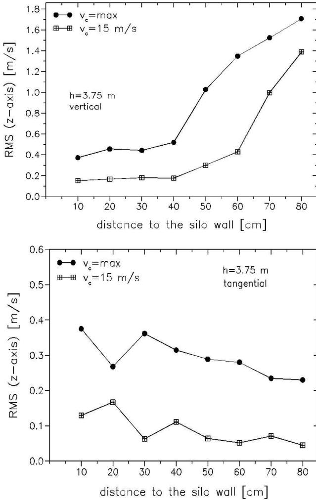
**Figure 5:** Influence of the conveying velocity on the RMS turbulent velocity of the particles filling the silo vertically (top) and tangentially (bottom)  $\xi=3 \text{ kg/m}^3$ .
