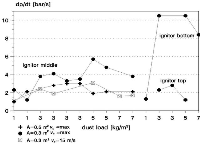
Figure 8: Pressure rate filling the silo pneumatically vertically with corn starch for two vent sizes and conveying velocities.
