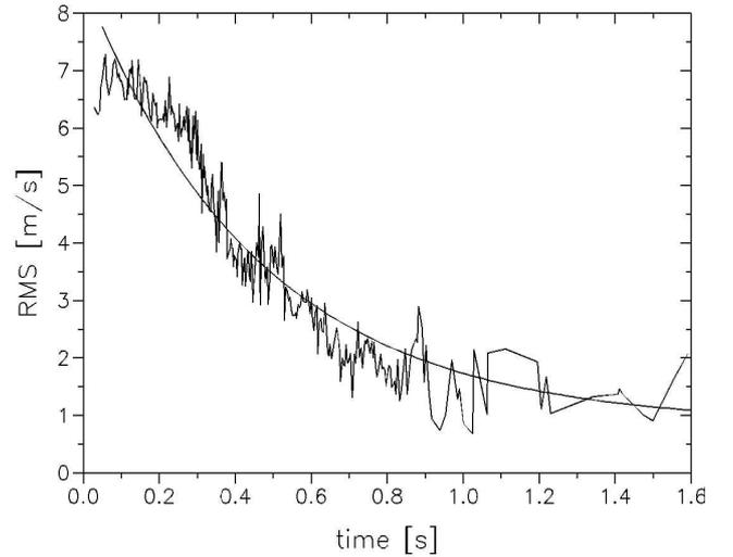
**Figure 3:** RMS turbulent velocity as a function of the time at the center of the 9.4 m<sup>3</sup>-silo with the regression curve according to  $RMS = 7.7 \cdot e^{-2.16 \cdot t} + 0.85$ . The dust was dispersed using ring nozzles.
