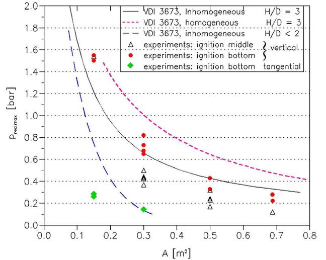
Figure 10: Comparison of the pressure–vent area course of the VDI 3673 guideline and our experimental results. The VDI-curves are calculated for a  $K_{St}$  of 140 bar m/s and  $p_{max}=9$  bar. The experimental data are only for a feeding rate of 3 and 5  $kg/m^3$  (maximum).
