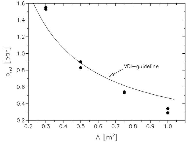
**Figure 6:** Reduced explosion-pressure measured as a function of the vent area for a ignition delay time of  $t_v=0.85 \text{ s}$  that is  $K_{\text{St}}=200 \text{ bar m/s}$ . The curve gives the results of the VDI-guideline 3673 for a homogeneous dust/air mixture.
