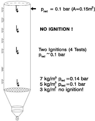
Figure 9: Survey of the single results at the different ignition positions using tangentially pneumatically filling. At a level of 3.75 m no ignition of the dust/air mixture was possible.
