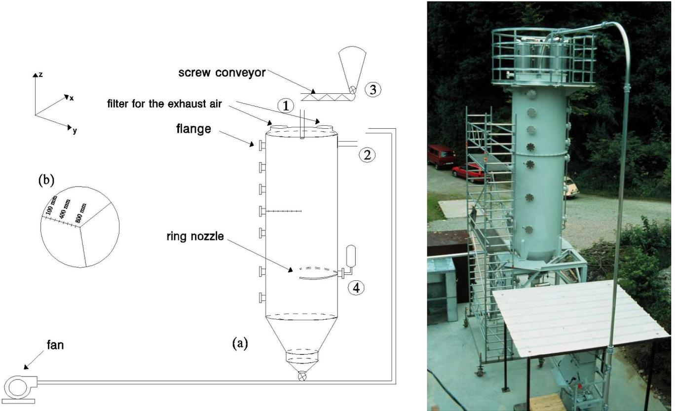
**Figure 1:** (a) Schematic diagram of the 12 m<sup>3</sup> (9.4m<sup>3</sup>)-silo. Four ways of feeding the silo are possible that are pneumatical vertical (1), pneumatical tangential (2), mechanical through a screw conveyor (3) and through four ring nozzle with pressurized dust chambers (4). The measuring probes were mounted at the different flanges. (b) shows the cross-section with the radial positions for the probes. On the right-hand side the practical realization is shown.
