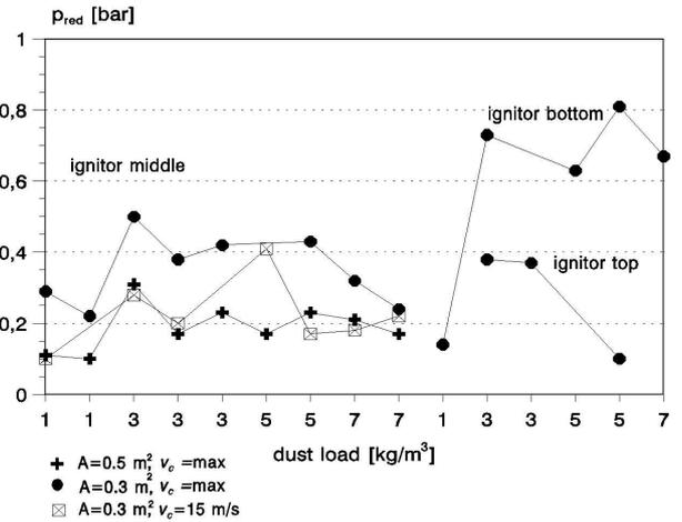
**Figure 7:** Reduced explosion-pressure after ignition filling the  $9.4 \text{ m}^3$ -silo pneumatically vertically with corn starch for two vent sizes and conveying velocities. The igniter was located at three different positions.
